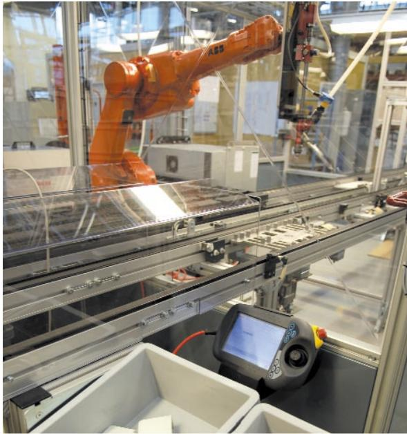
cell uses one IRB 1600 robot to automatically mount screws in the unit. According to Persson, the line is capable of assembling one fuse switch disconnecter per minute and has substantially increased Kabeldon's productivity. Previous assembly was done manually at four different workstations, which obviously took more time and required more floor space. "Another benefit is that the quality of the units has noticeably improved," says Persson.
